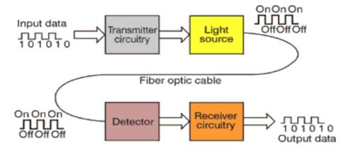
Figure 1: Basic fiber optic communication system [29]
