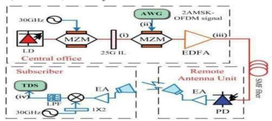
Fig. 6. Experimental setup of the proposed scheme (MZM: Mach-Zehnder
