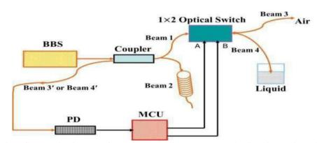
Fig.7. Schematic diagram of RI sensor system based on the  $1 \times 2$  optical switch [48].
